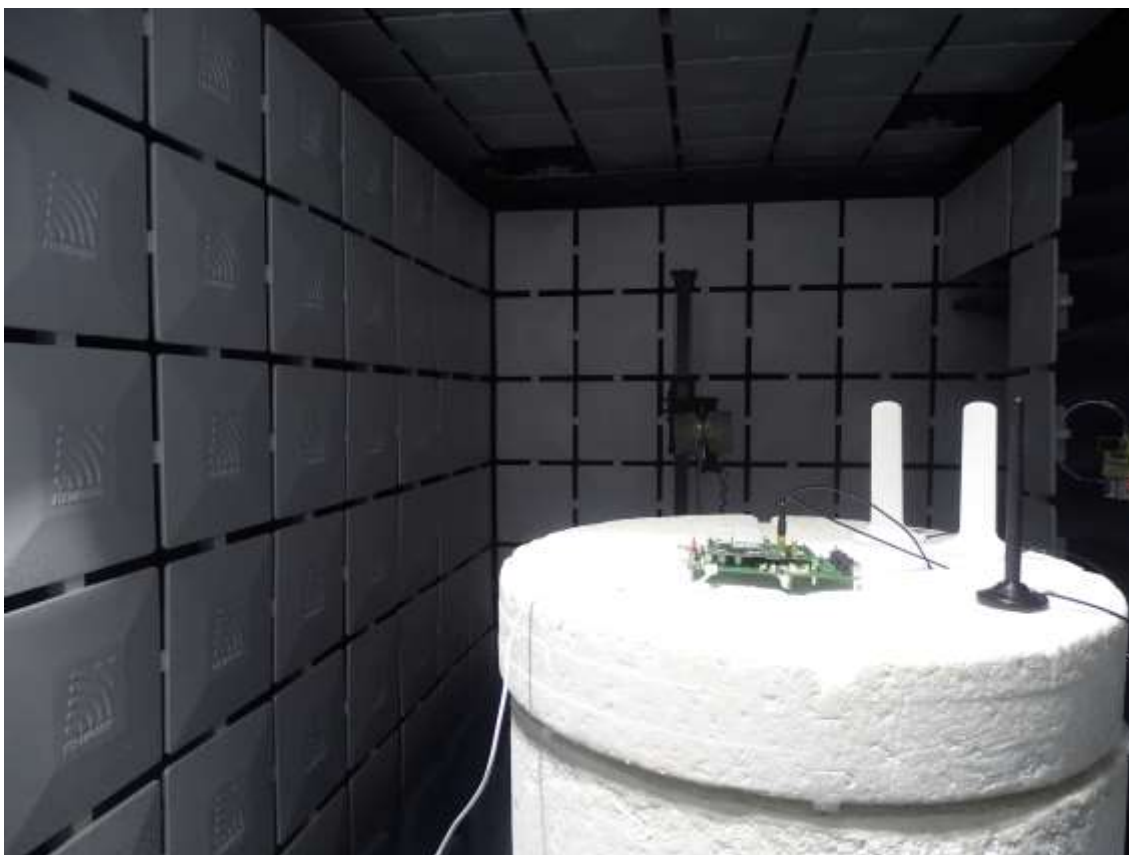
Radiated Spurious Emission (3GHz to18GHz)
