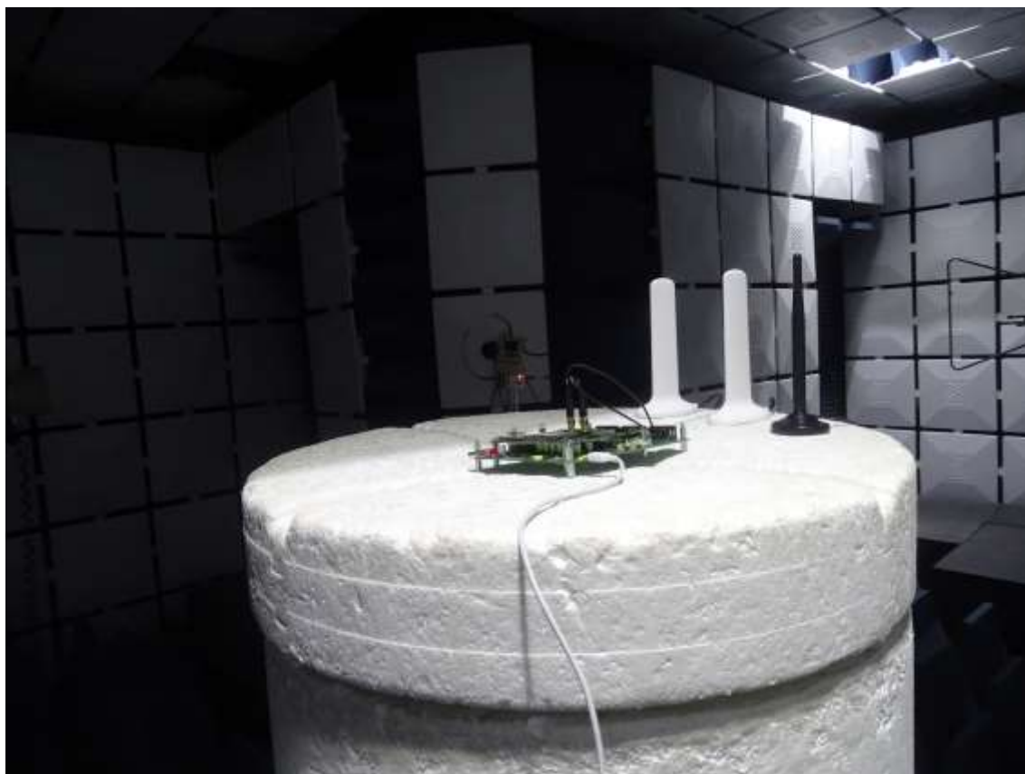
Radiated Spurious Emission (18GHz to26.5GHz)
