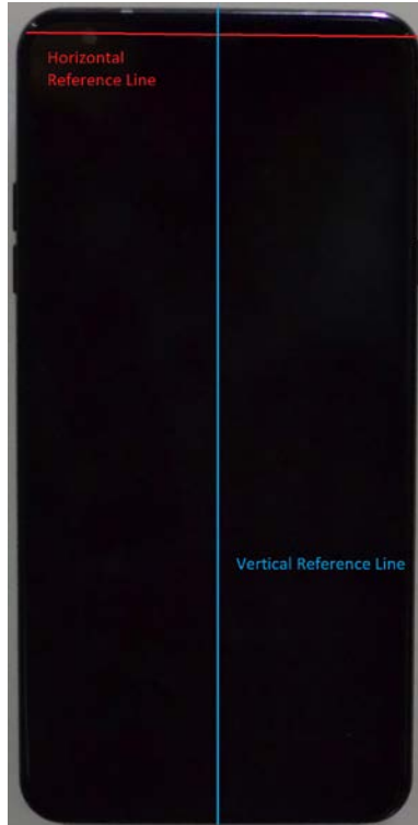
SAR Test Setup Photo 17: Vertical and Horizontal Reference Lines
