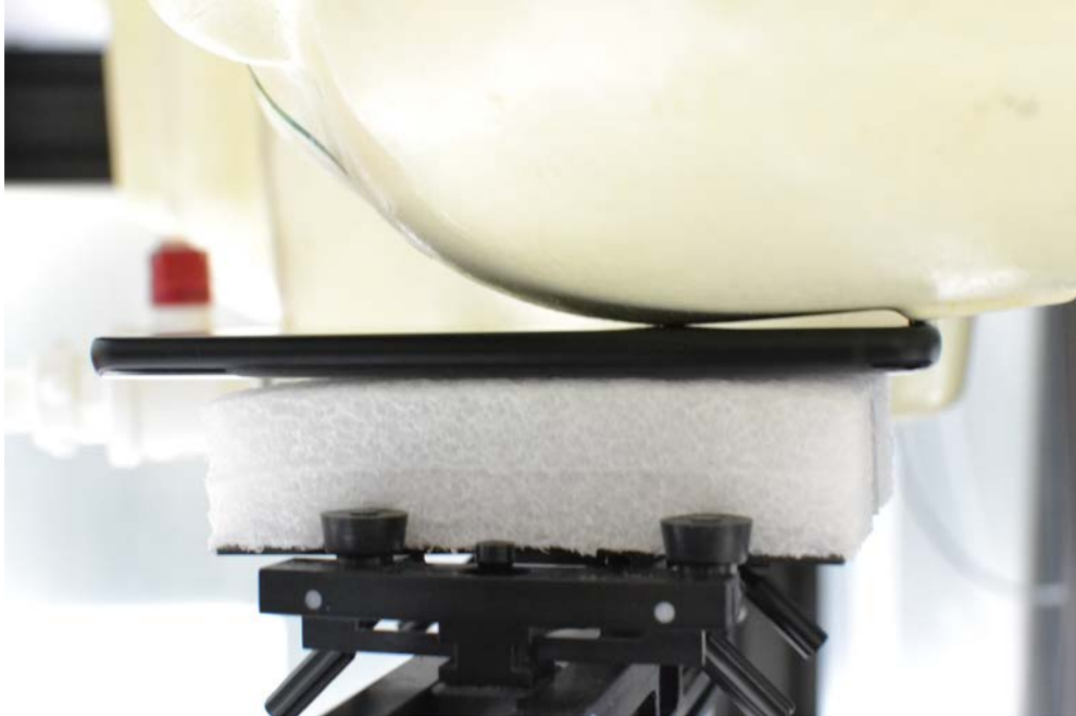
SAR Test Setup Photo 3: Left Cheek
