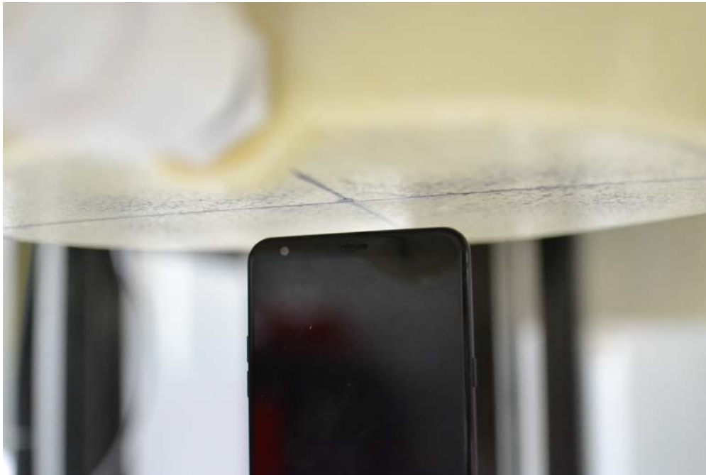
SAR Test Setup Photo 11: Top Edge at 1.0 cm
