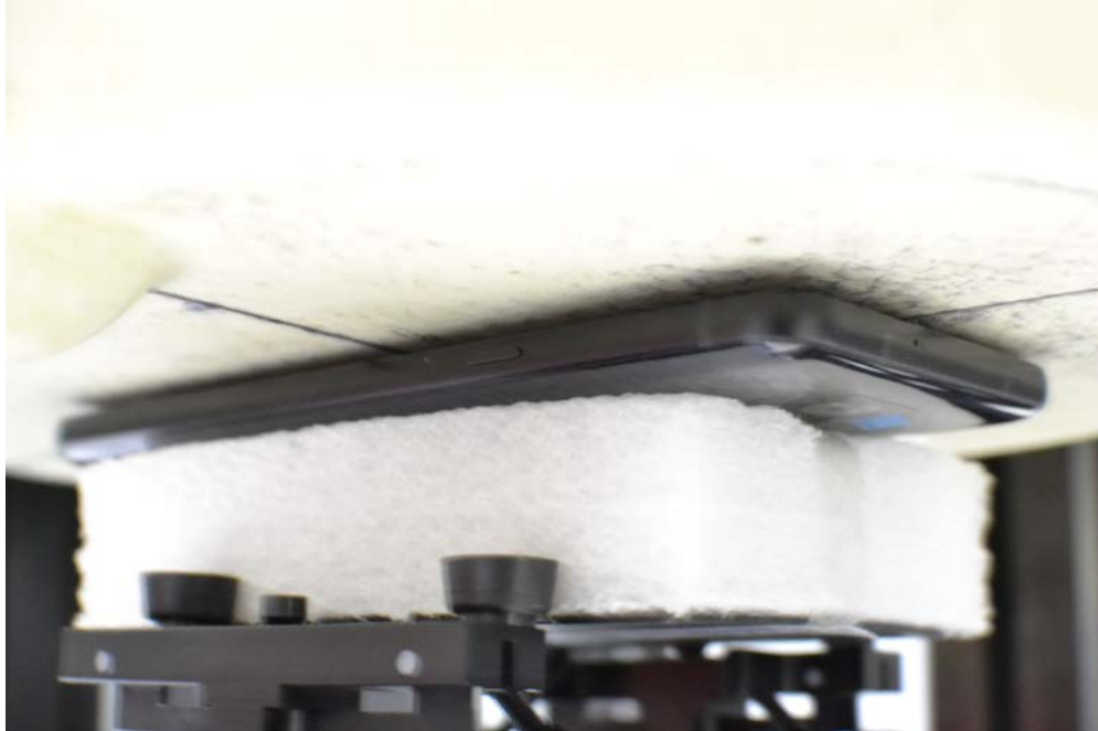
SAR Test Setup Photo 9: Front Side at 0.2 cm
