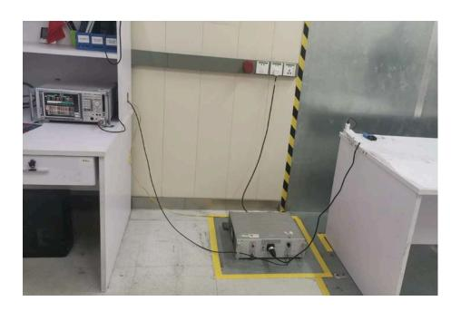
Spurious Emission Test Setup (Below 1GHz)
