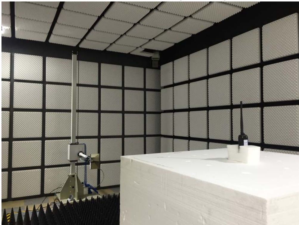
Radiated RF measurement (Above 1 GHz)
