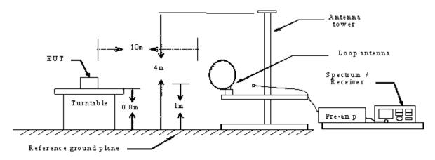
Radiated Spurious Measurement: below 1GHz
