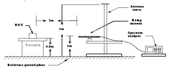
Radiated Spurious Measurement: above 1GHz
