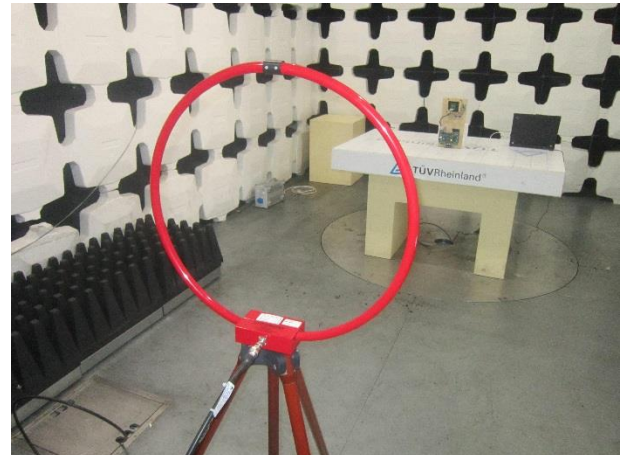
Set-up radiated emission test
