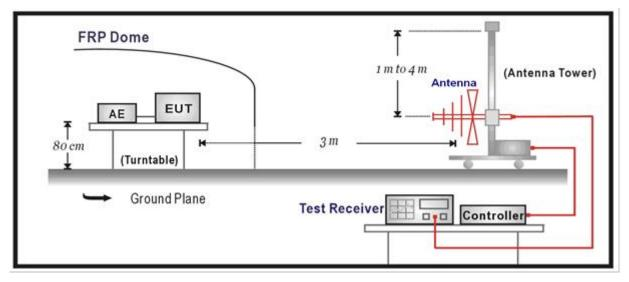
Above 1GHz Test Setup:
