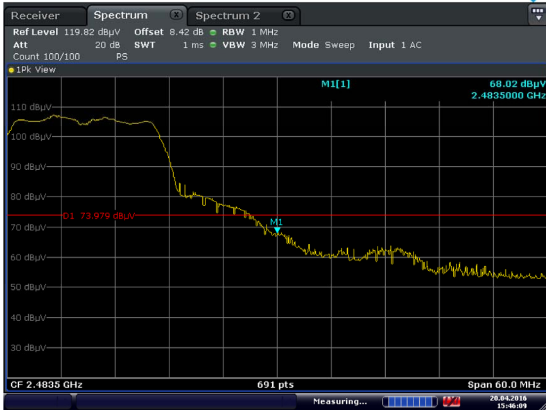
Plot 7-54. Radiated Restricted Upper Band Edge Measurement (Peak)
