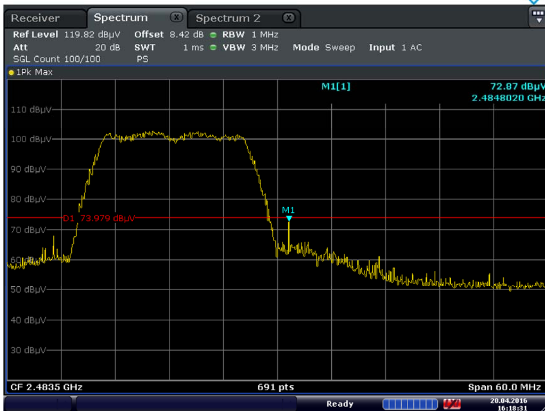
Plot 7-58. Radiated Restricted Upper Band Edge Measurement (Peak)
