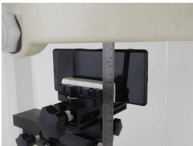
Right Side, Test Separation 10 mm
