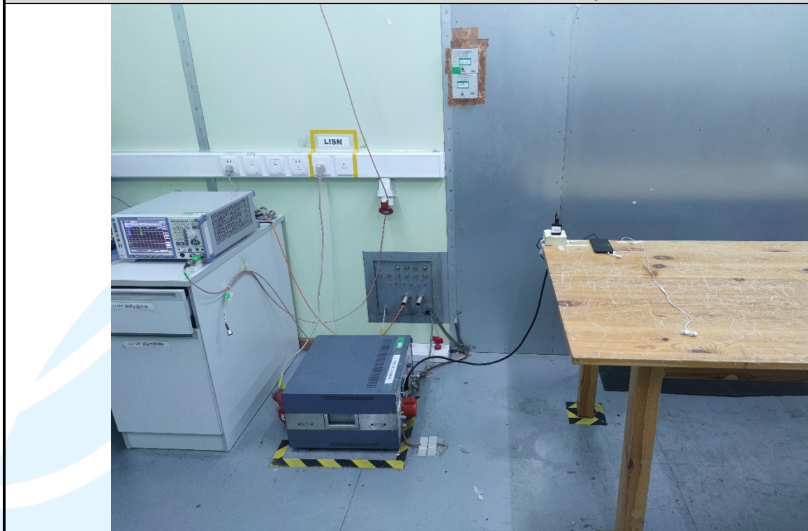
Conducted Emission Test Setup
