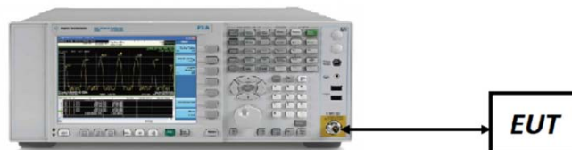
Figure 7-1. Test Instrument & Measurement Setup
