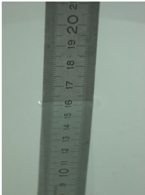
Fig. 31: Liquid depth (16.2 mm) for the GSM 1900 Body measurements.
