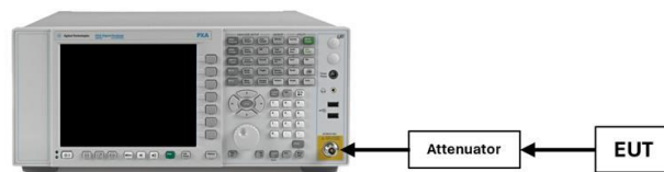
Figure 7-3. Test Instrument & Measurement Setup
