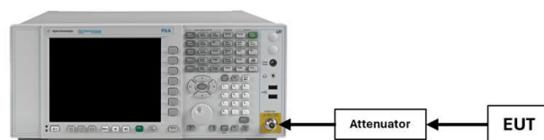
Figure 7-4. Test Instrument & Measurement Setup
