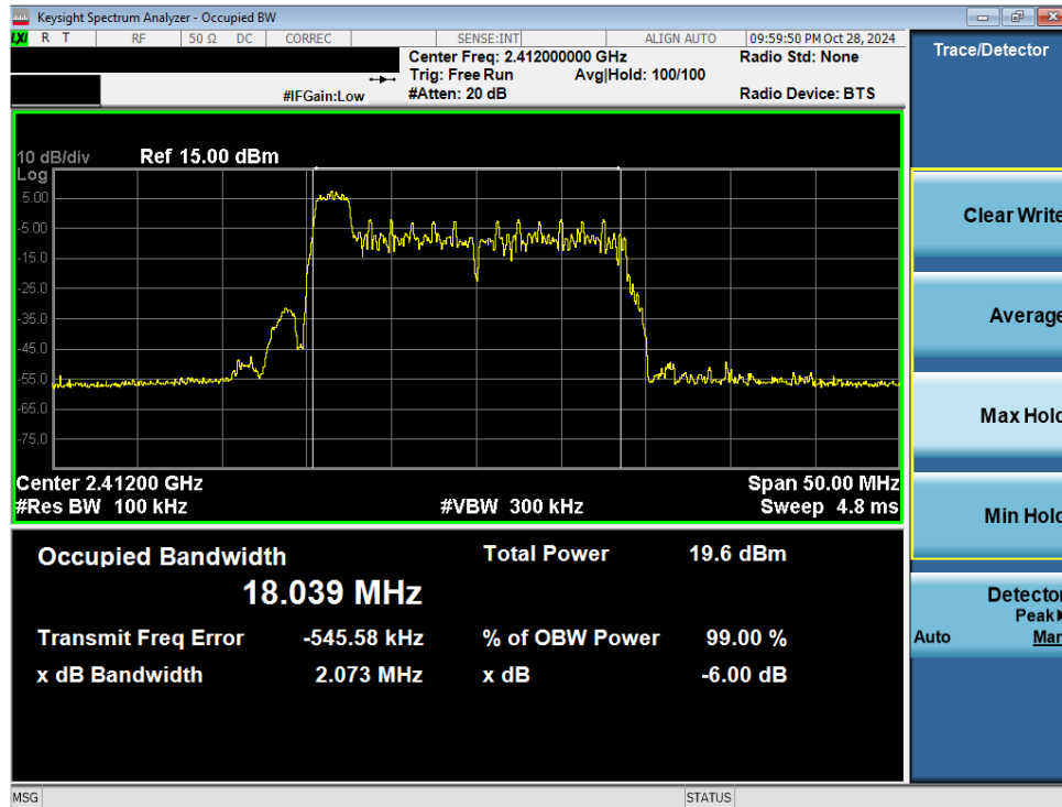
Plot 7-5. 6dB BW & 99% OBW Antenna WF7b (802.11ax OFDMA – RU26 – Ch. 1)
