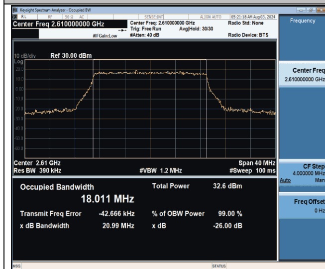
Band38-20MHz-QPSK-38150-100RB#0-PASS
