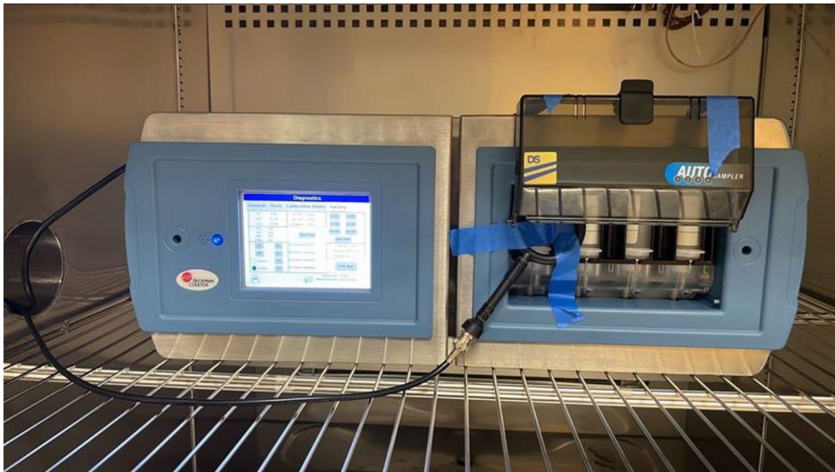
CONDUCTED EUT OBW & FREQUENCY STABILITY SETUP
