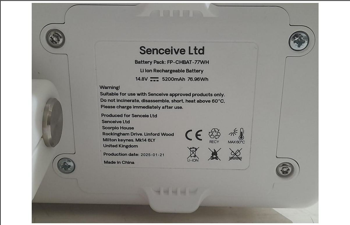
Camera Hub FM3C-LTE (CH) – Battery Pack Enclosure Cover with Battery Pack Details
