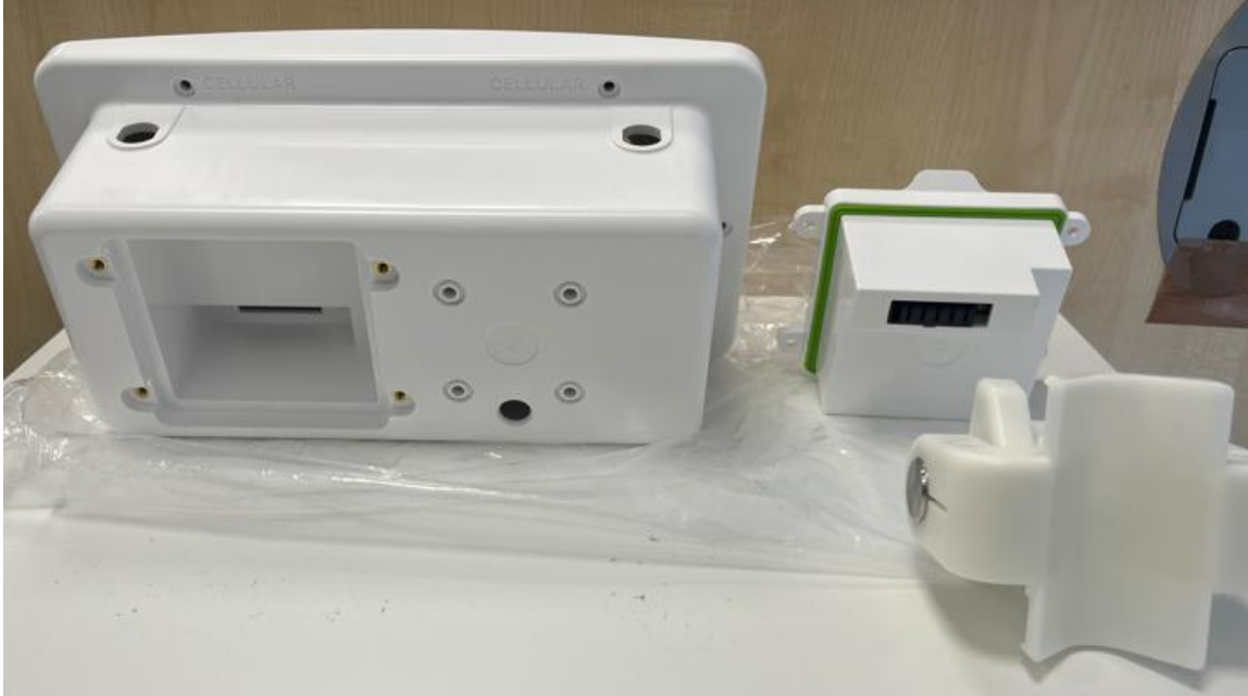
Camera Hub FM3C-LTE (CH) Rear View with both Battery Pack and fixing bracket removed
