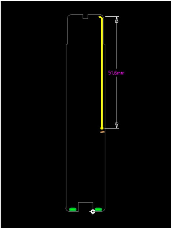
Antenna located on the top view of PCB
