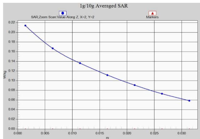
Fig.3 Z-Scan at power reference point (LTE Band5)
