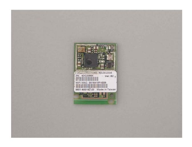
Top View "Transmitter Board, Shield Removed"
