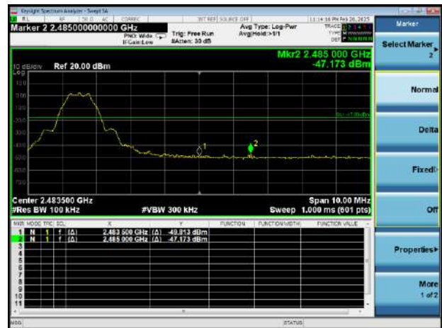
GFSK (BLE 1Mbps) HIGH CHANNEL, BAND EDGE
