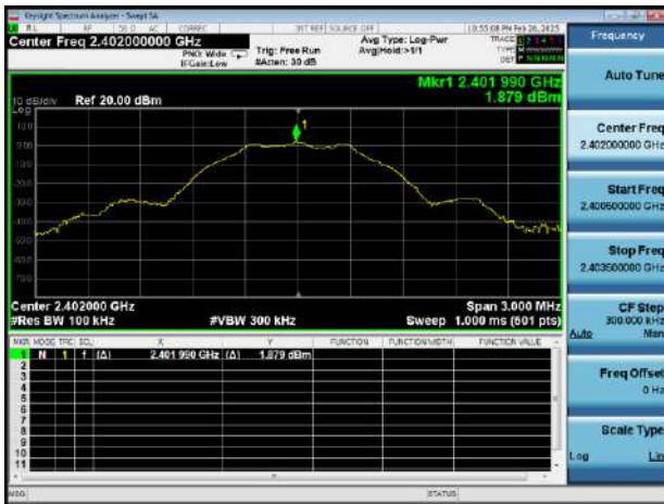
GFSK (BLE 1Mbps) LOW CHANNEL, CARRIER LEVEL
