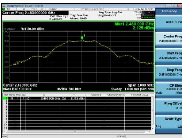
GFSK (BLE 1Mbps) HIGH CHANNEL, CARRIER LEVEL
