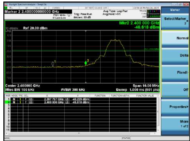
GFSK (BLE 1Mbps) HIGH CHANNEL, BAND EDGE
