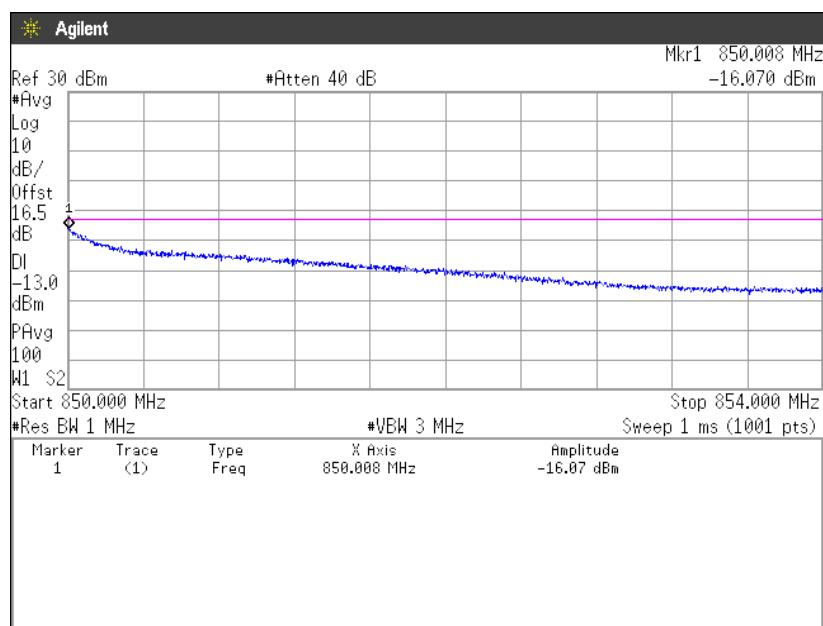
**(Spurious Emissions)****Note: Conducted spurious test was measured in the worst case of conducted output power.****Channel: 4132**
