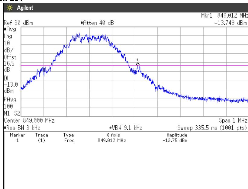
**(Spurious Emissions)****Note: Conducted spurious test was measured in the worst case of conducted output power.****Channel: 128**
