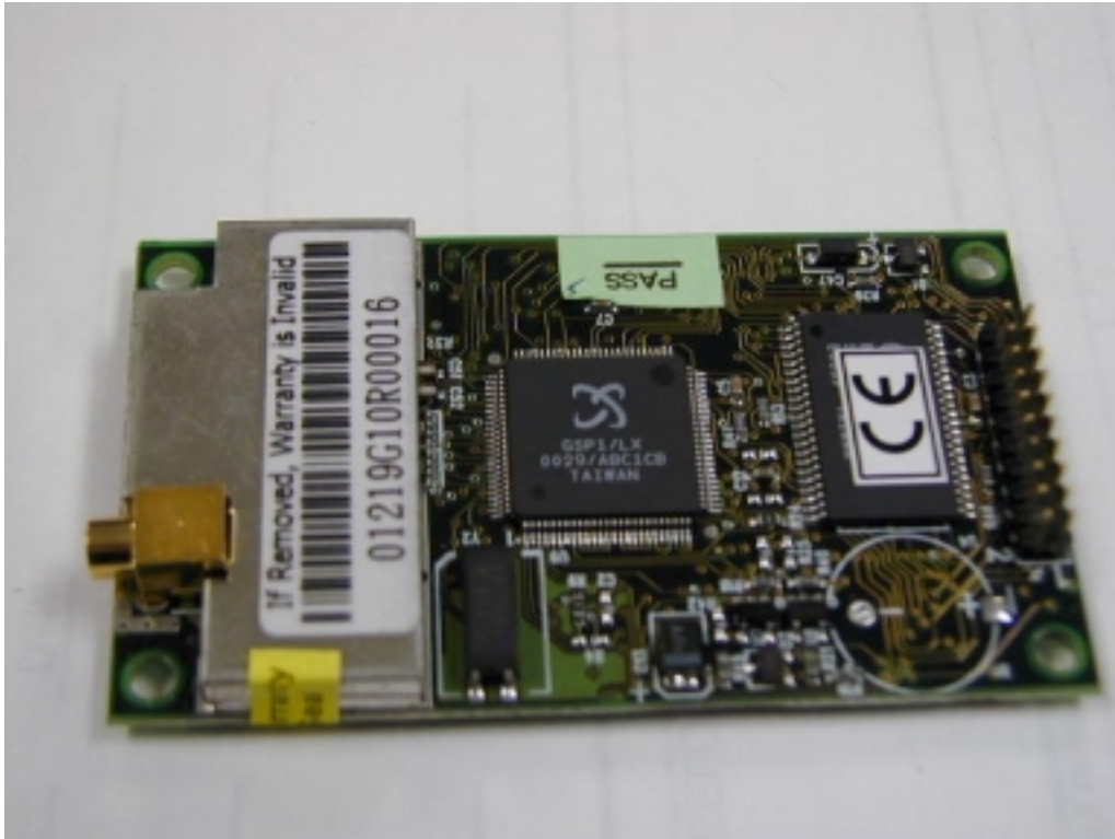
GPS receiver board, side 2 (above).
