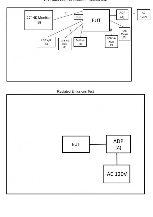
AC Power Line Conducted Emissions Test
