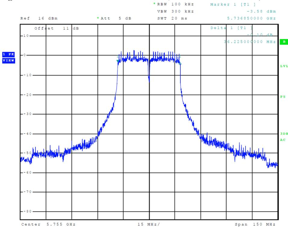
**Figure 22 Plot of Transmitter Emissions (5725-5850 MHz Band, 802.11n40, 6-dB OBW)**
