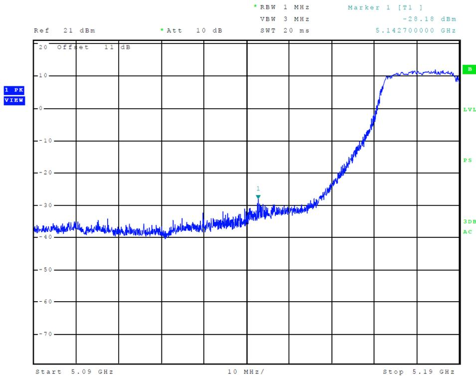
**Figure 6 Plot of Transmitter Low Band Edge (5150-5250 MHz Band, 802.11n40)**
