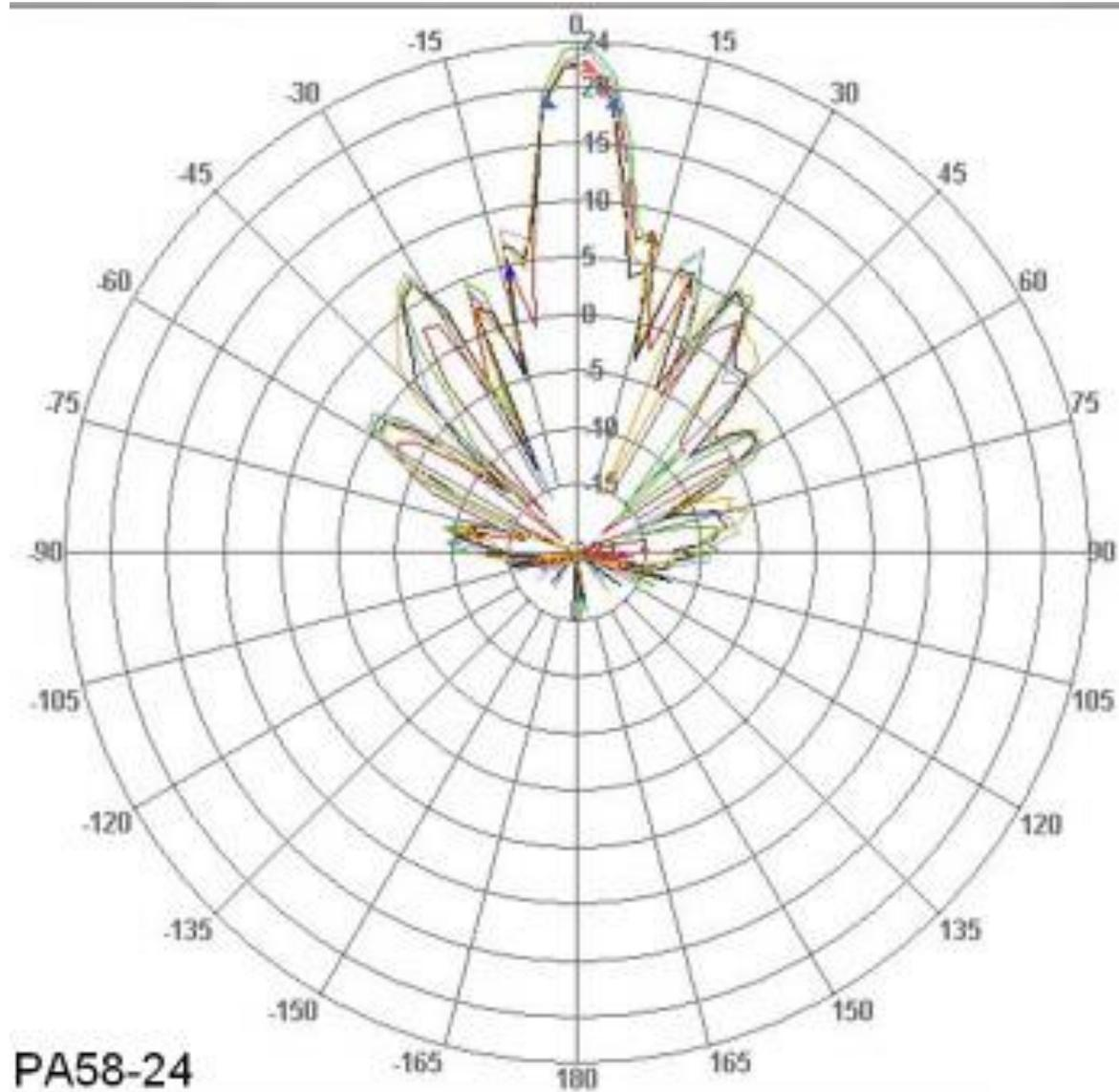
**Elevation Compliance Dish Antenna (32 dBi) HDDA5W-32-DP2**
