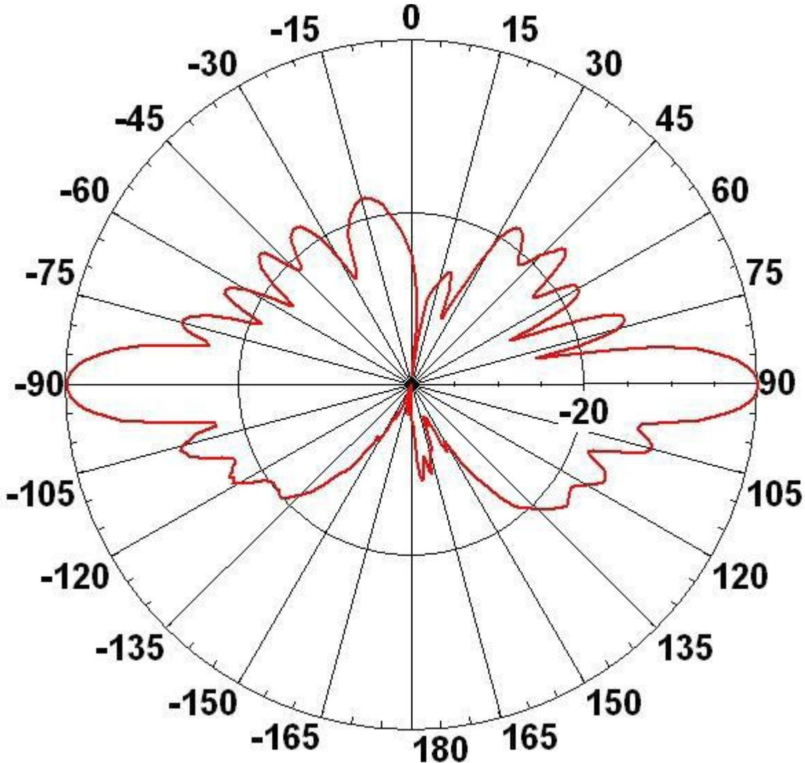
**Elevation Compliance Panel Antenna (24 dBi) PA58-24-ANT**
