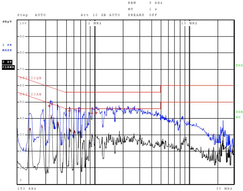
**Figure 1 AC Line Conducted Emissions Line 1**
