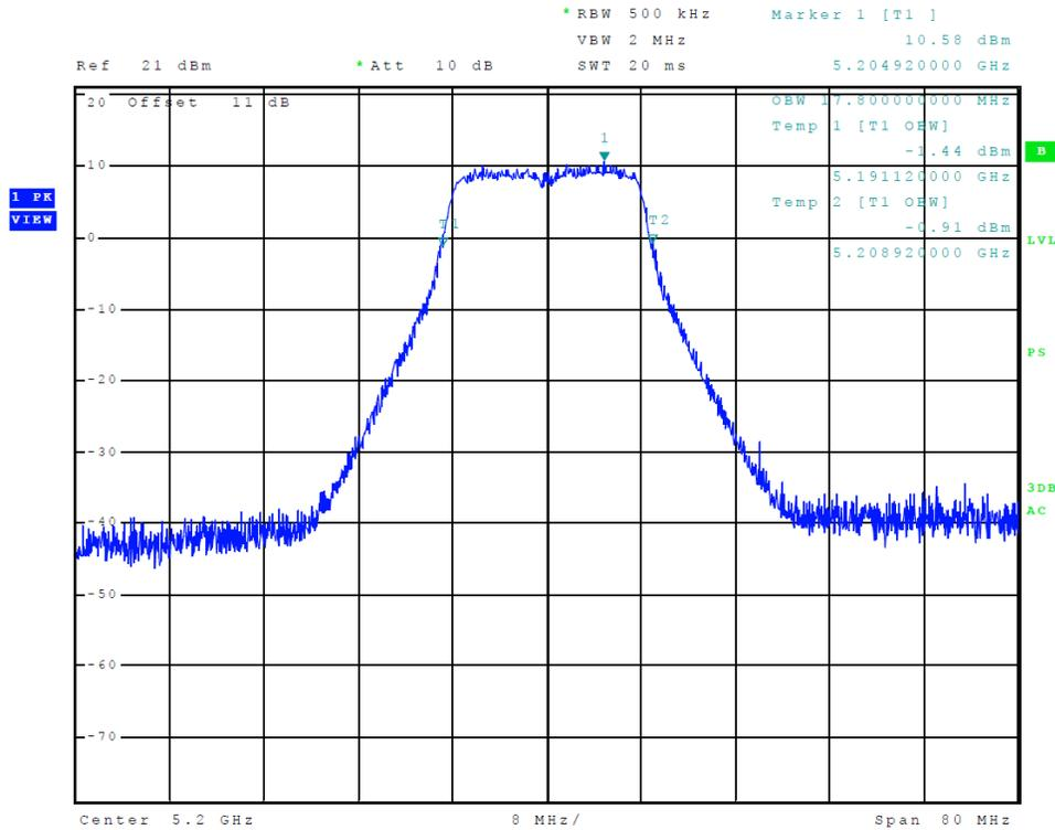
**Figure 9 Plot of Transmitter Emissions (5150-5250 MHz Band, 802.11a, 99% OBW)**
