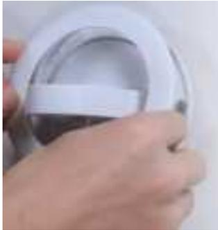
Step 6. Install the Extender into the bracket and connect the AC adapter to the Extender's DC jack.
