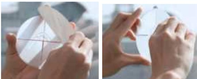
Step 4. To eliminate air bubbles use both thumbs to press in all areas where the Gecko adhesive pad contacts the glass. Press for one minute (30 seconds on the upper part and 30 seconds on the lower part).
