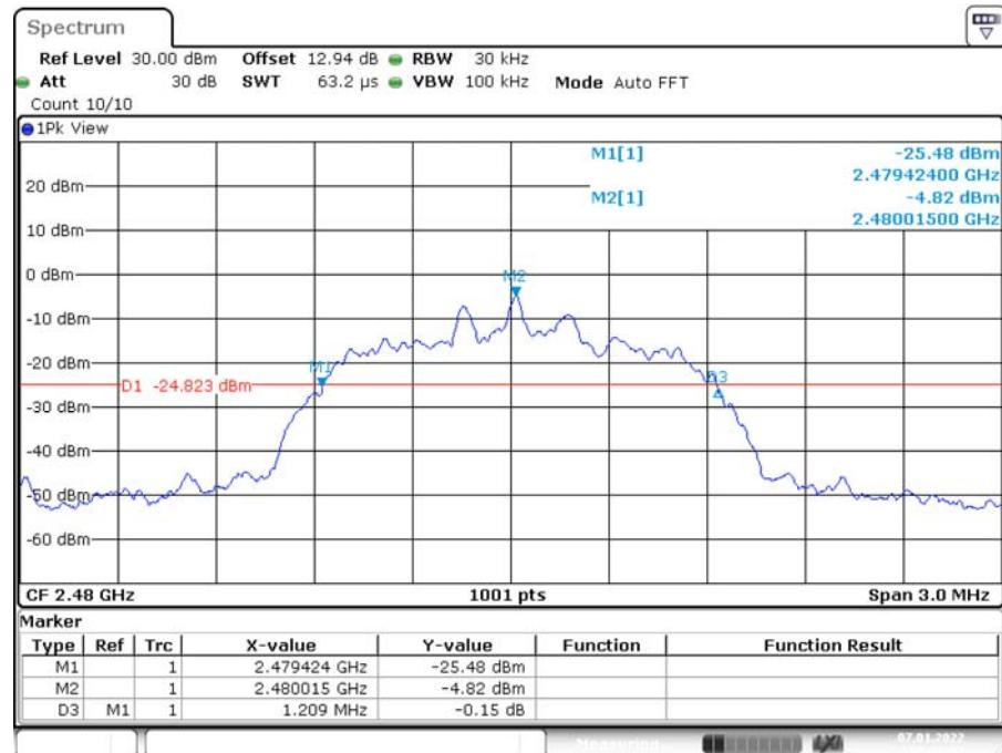
**99% OCCUPIED BANDWIDTH****DH1\_Ant1\_2402MHz**
