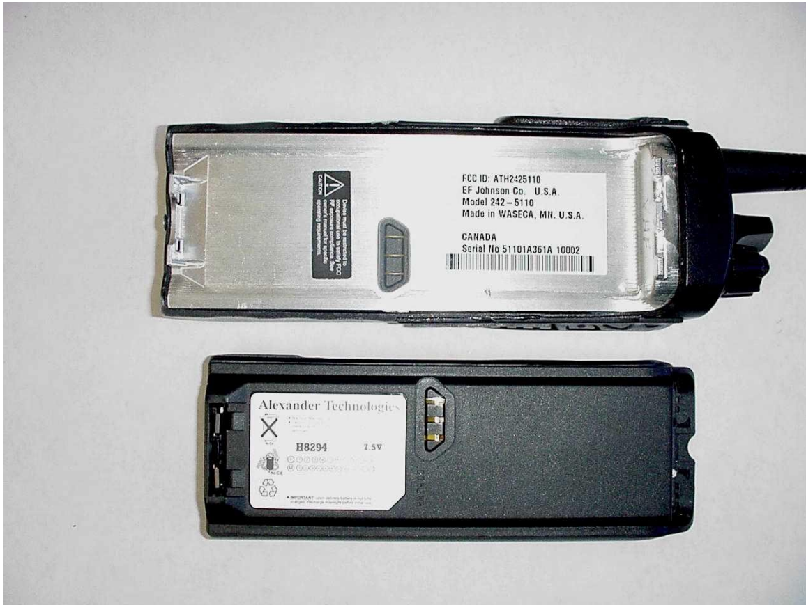
PHOTOGRAPH 8: RADIO BACK VIEW – BATTERY REMOVED
