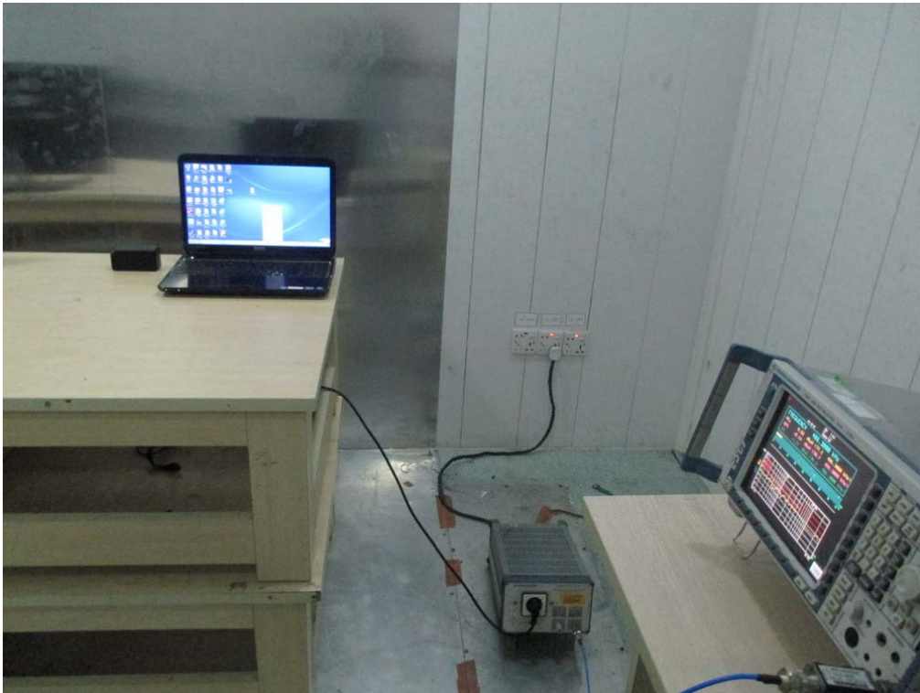
FCC RADIATED EMISSION TEST SETUP
