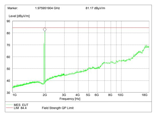
Note: The emission close to the limit is the operating frequency.
