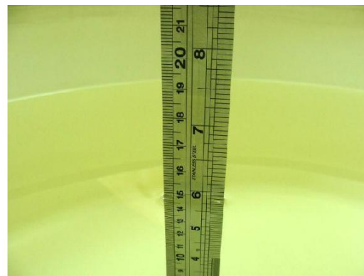
Fig 7.2 Photo of Liquid Height for Body SAR
