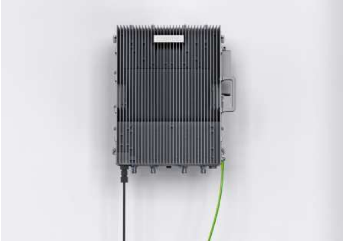
Figure 37. Connect the Grouding Cable of E62-X3
