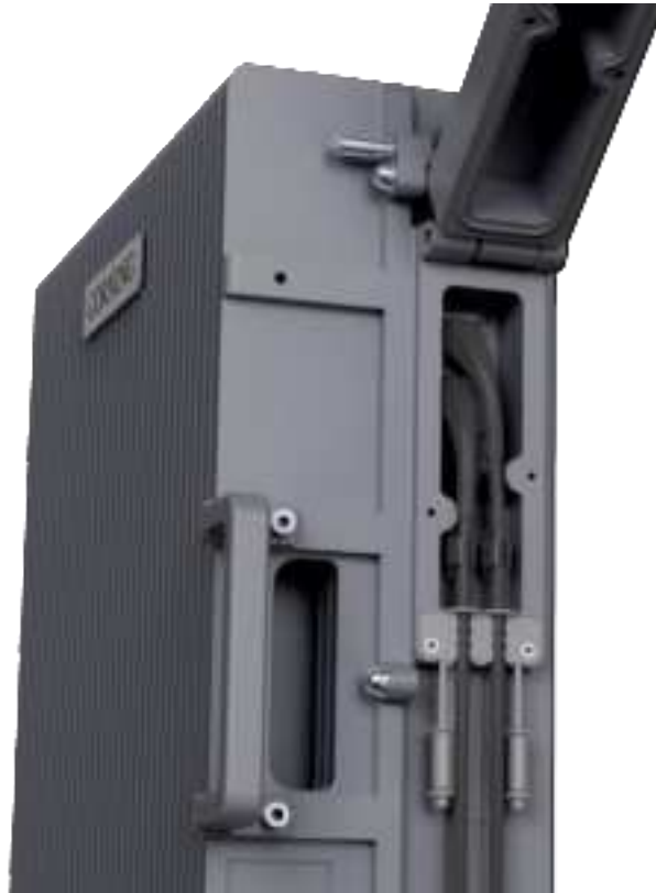
Figure 49. Open the Box and connect the SFP
