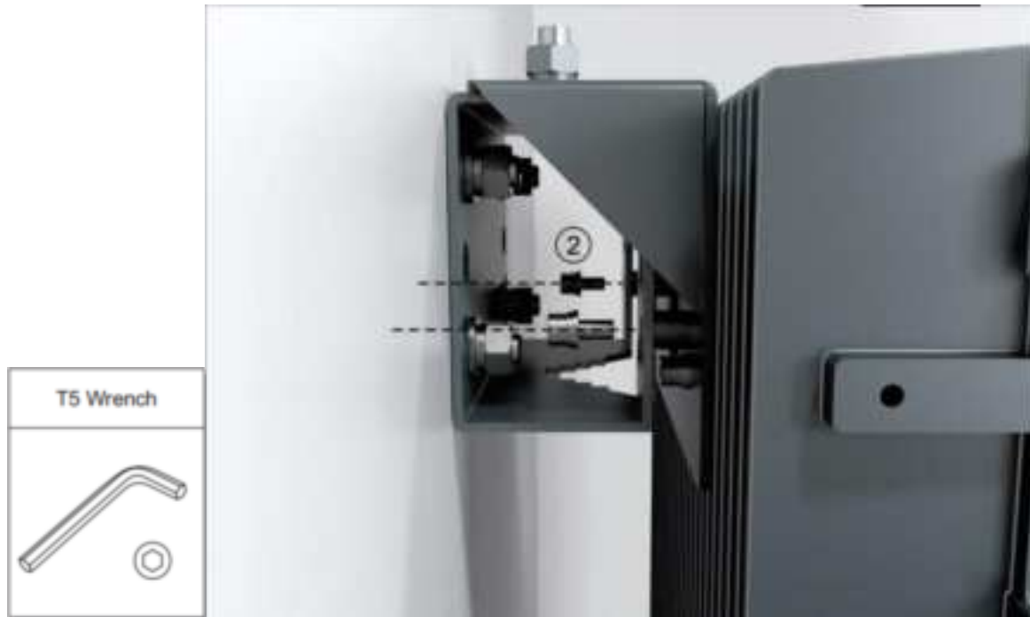
Figure 35. Fasten the Bracket I and II
