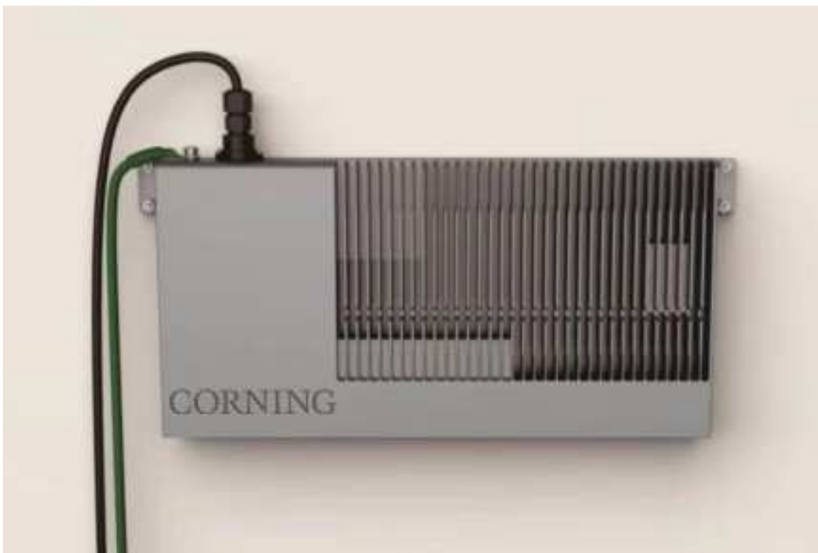
Figure 26. E3 Wall Mounting Completed
