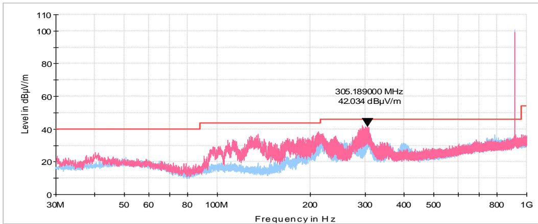
**Plot 7.2.6 Radiated emission measurements from 30 to 1000 MHz**
