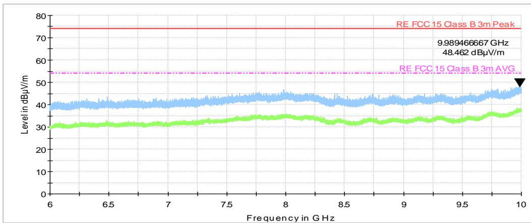
**Plot 7.2.12 Radiated emission measurements from 6 to 10 GHz**
