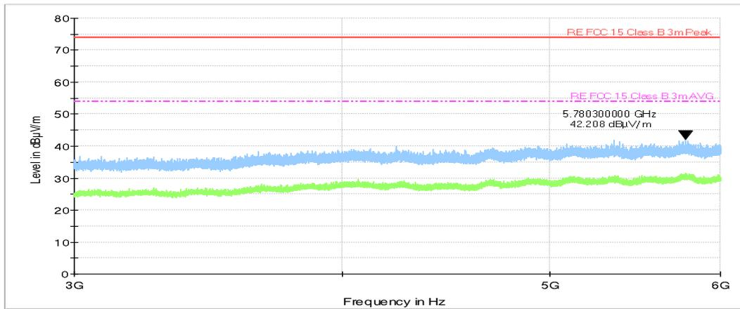
**Plot 7.2.10 Radiated emission measurements from 3 to 6 GHz**
