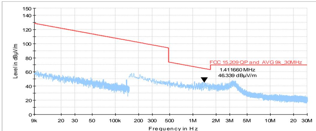
**Plot 7.2.4 Radiated emission measurements from 9 kHz to 30 MHz**
