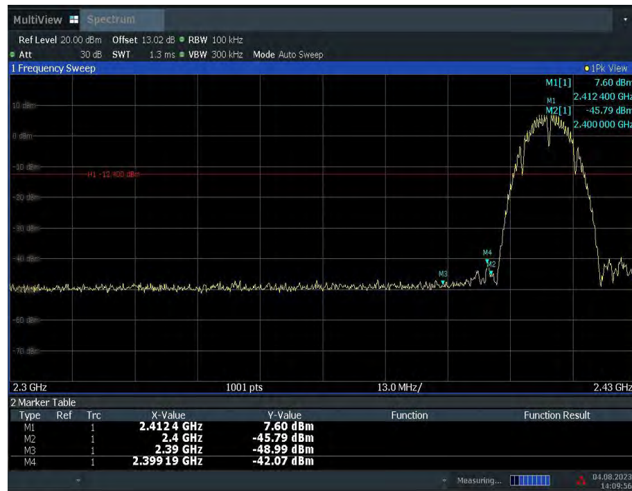
Fig.A.5.1 Band Edges (802.11b, Ch 1)
