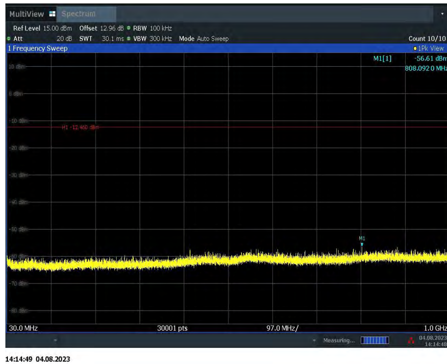
Fig.A.6.1.5 Transmitter Spurious Emission - Conducted (802.11b, Ch6, 30 MHz-1 GHz)
