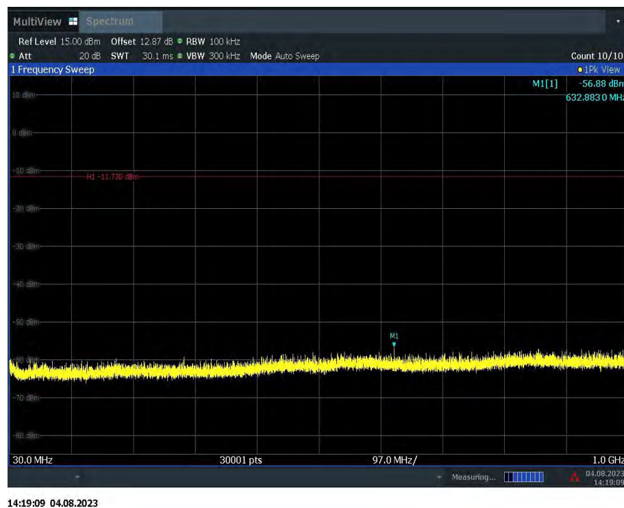
Fig.A.6.1.8 Transmitter Spurious Emission - Conducted (802.11b, Ch11, 30 MHz-1 GHz)
