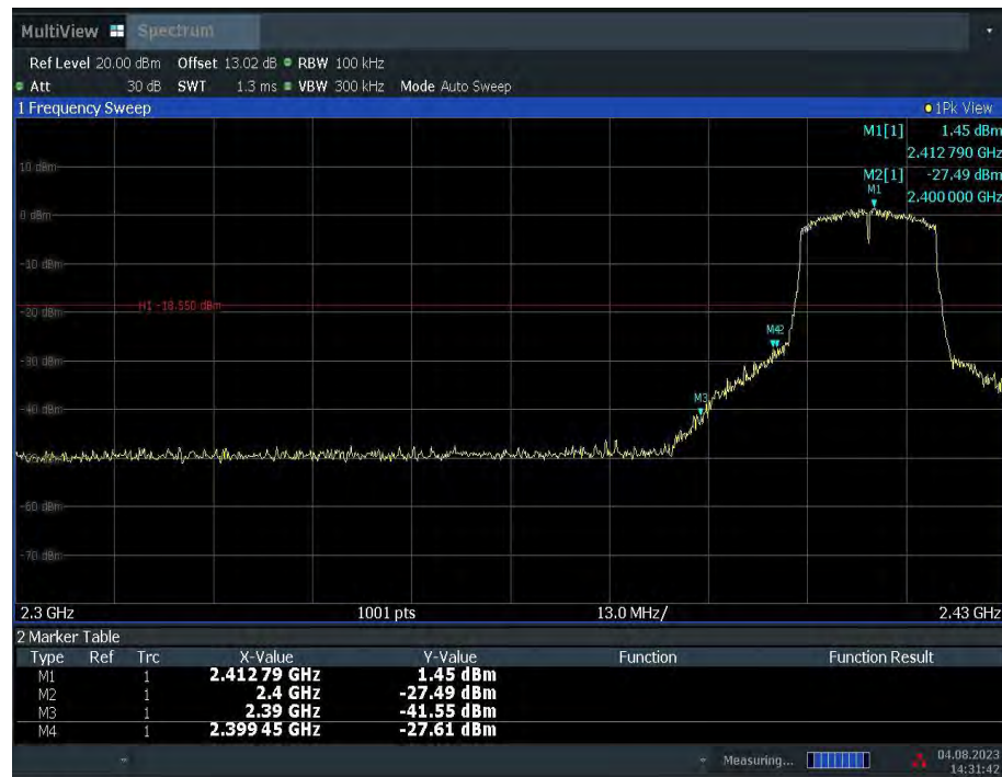
Fig.A.5.5 Band Edges (802.11n-HT20, Ch 1)
