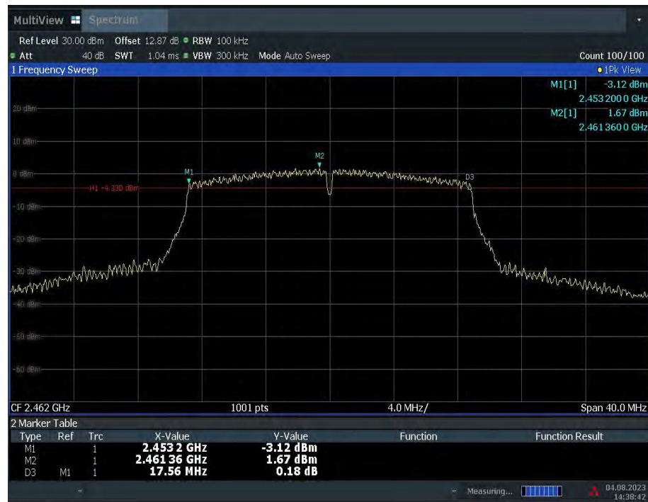
Fig.A.4.9 Occupied 6dB Bandwidth (802.11n-HT20, Ch 11)
