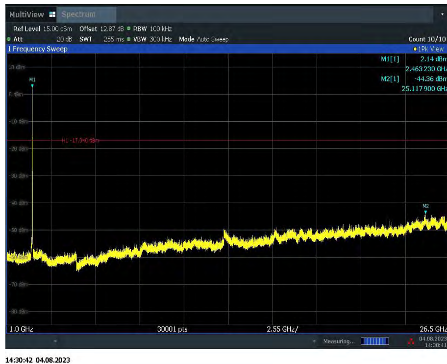
Fig.A.6.1.18 Transmitter Spurious Emission - Conducted (802.11g, Ch11, 1 GHz-26.5 GHz)
