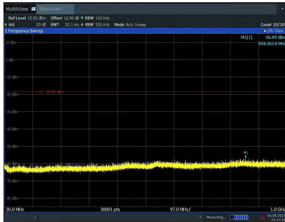
Fig.A.6.1.23 Transmitter Spurious Emission - Conducted (802.11n-HT20, Ch6, 30 MHz-1 GHz)
