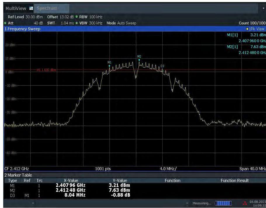
Fig.A.4.1 Occupied 6dB Bandwidth(802.11b,Ch 1)
