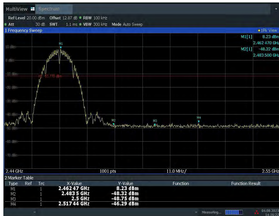
Fig.A.5.2 Band Edges (802.11b, Ch 11)
