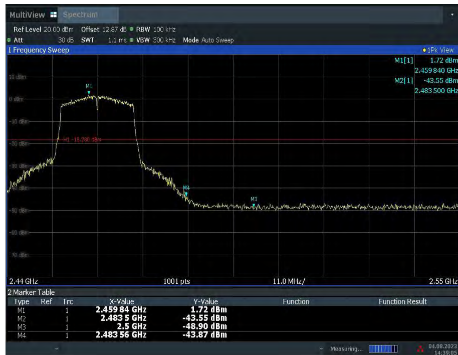
Fig.A.5.6 Band Edges (802.11n-HT20, Ch 11)
