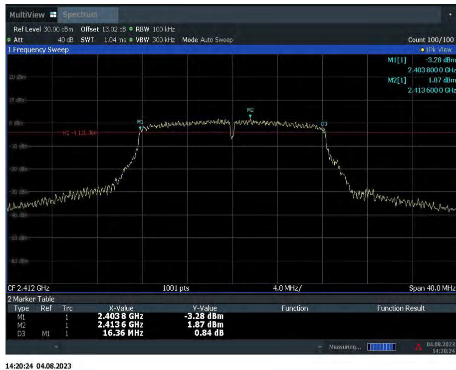
Fig.A.4.4 Occupied 6dB Bandwidth (802.11g, Ch 1)
