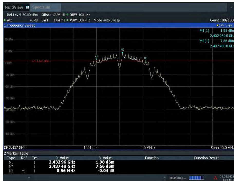
Fig.A.4.2 Occupied 6dB Bandwidth (802.11b, Ch 6)
