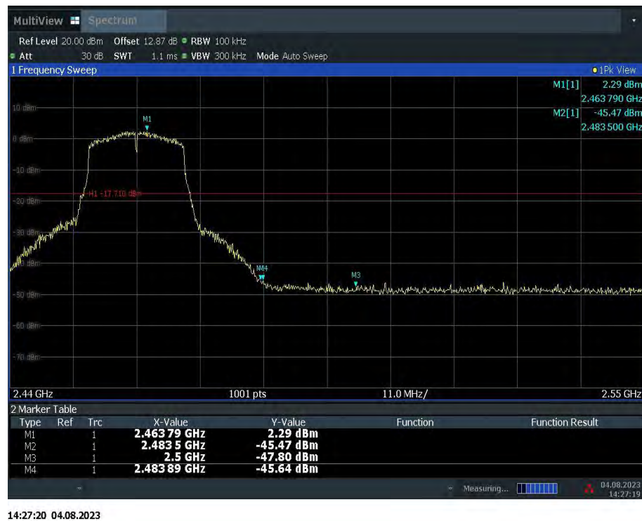
Fig.A.5.4 Band Edges (802.11g, Ch 11)
