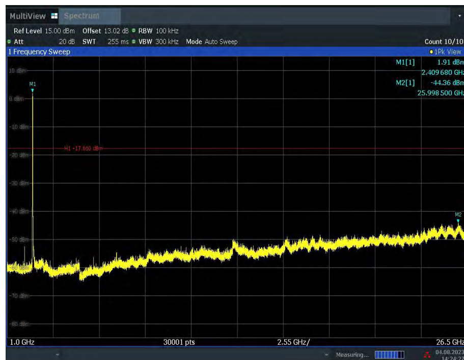
Fig.A.6.1.12 Transmitter Spurious Emission - Conducted (802.11g, Ch1, 1 GHz-26.5 GHz)
