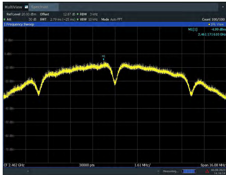
Fig.A.3.3 Power Spectral Density (802.11b, Ch 11)
