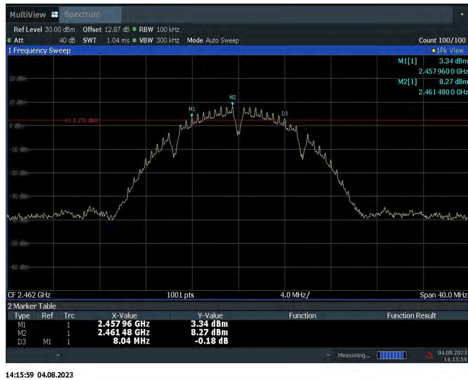
Fig.A.4.3 Occupied 6dB Bandwidth (802.11b, Ch 11)
