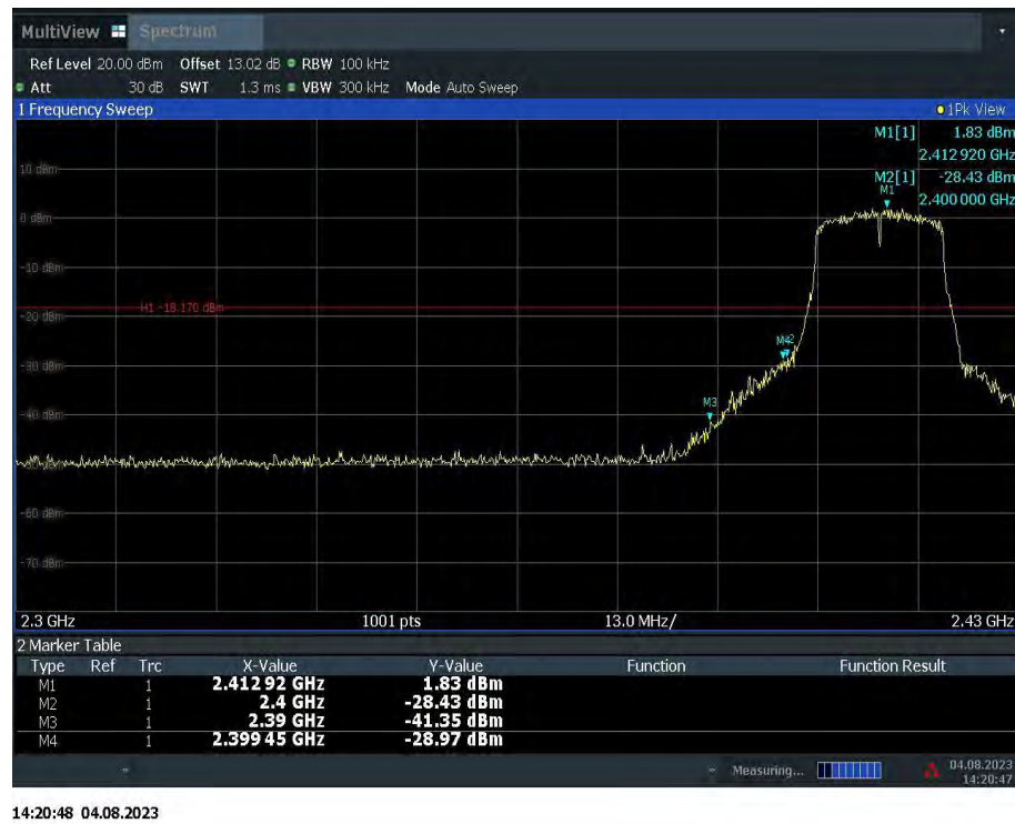
Fig.A.5.3 Band Edges (802.11g, Ch 1)
