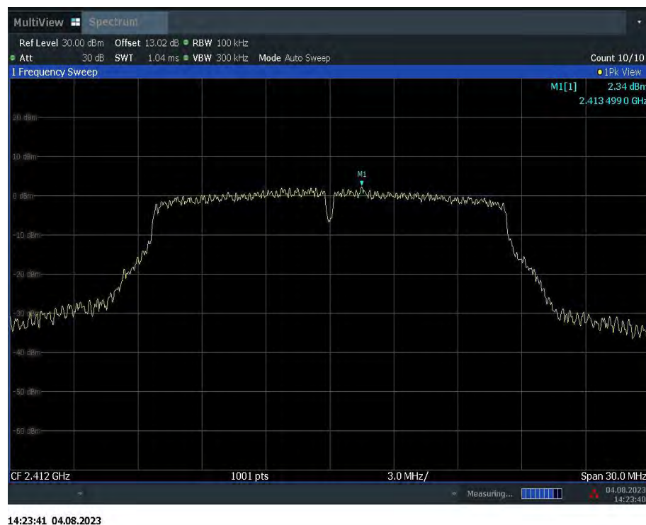
Fig.A.6.1.10 Transmitter Spurious Emission - Conducted (802.11g, Ch1, Center Frequency)
