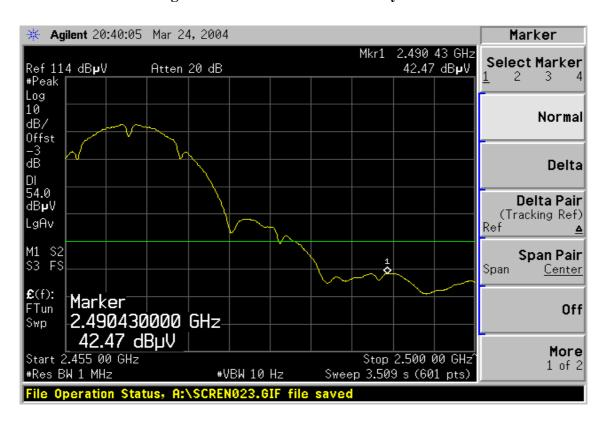
Detector mode: Peak Polarity: Horizontal
