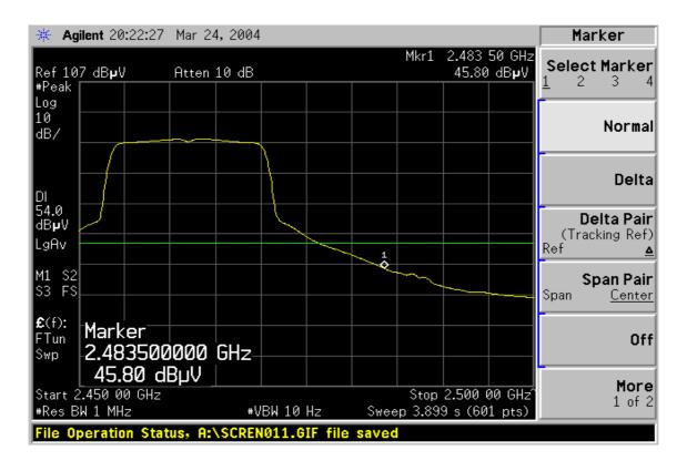
Detector mode: Peak Polarity: Horizontal
