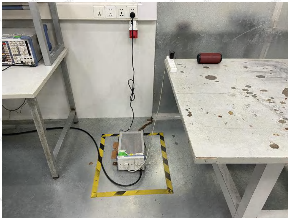
Photo of Conducted Emission Measurement
