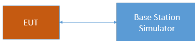
Test Setup FCC Part 22/24/27/90 Cellular; Frequency stability
