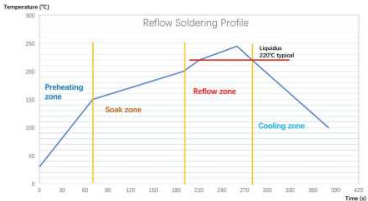
Figure 19: Temperature-Time Profile for Reflow Soldering
