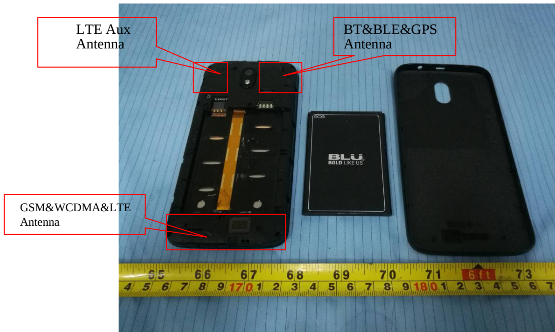
EUT – Cover off View 1
