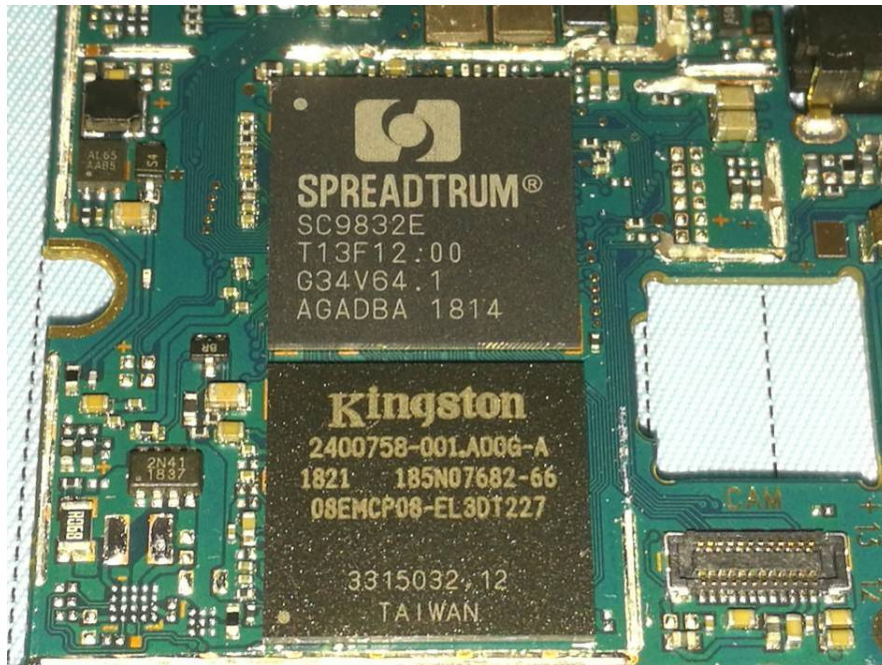
EUT – Main Chip 2 View
