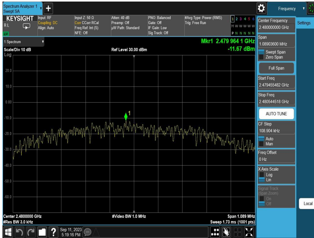
Plot 7-9. Power Spectral Density Plot (Bluetooth (LE), 1Mbps – Ch. 39)
