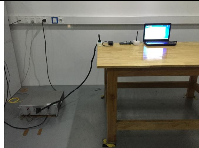
Conducted Emissions Test Setup Front View
