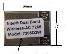
Manufacturer & model number will appear on module for identification. Label will be replaced with laser etching on the metal shield for high volume manufacturing.
