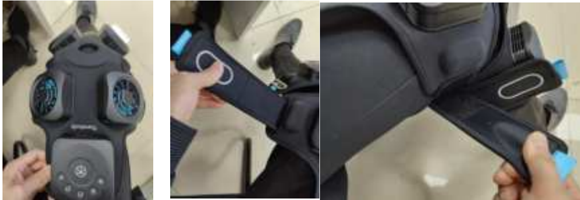
Fig. 1.1 Align knee with the central hole Fig. 1.2 Strap passes through the hole buckle Fig. 1.3 Stick the velcro tight
