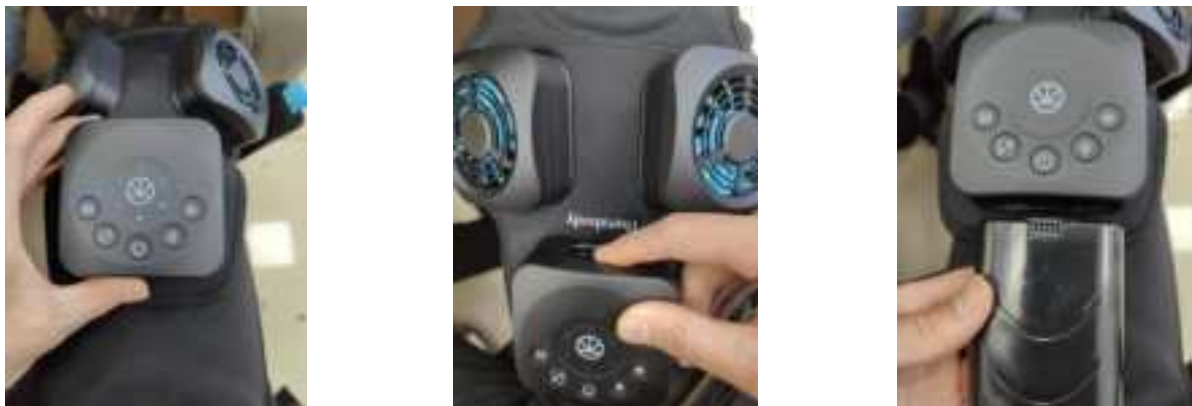
Figure 2.1 Insert the battery with the electrode facing up Figure 2.2 Power on self inspection Figure 2.3 Push out the battery
