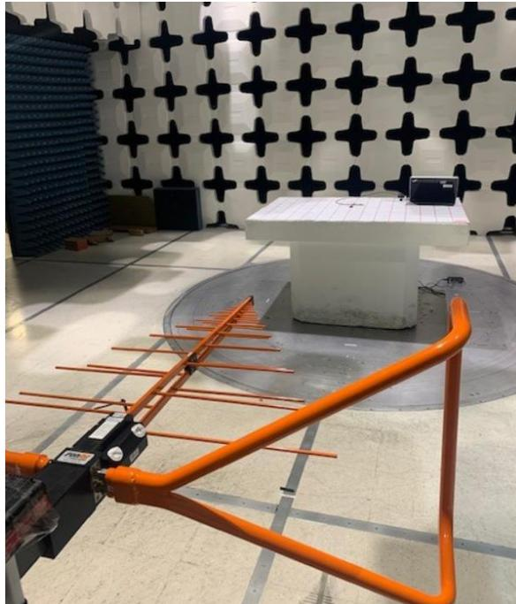
Radiated Emission Test below 1GHz Front View
