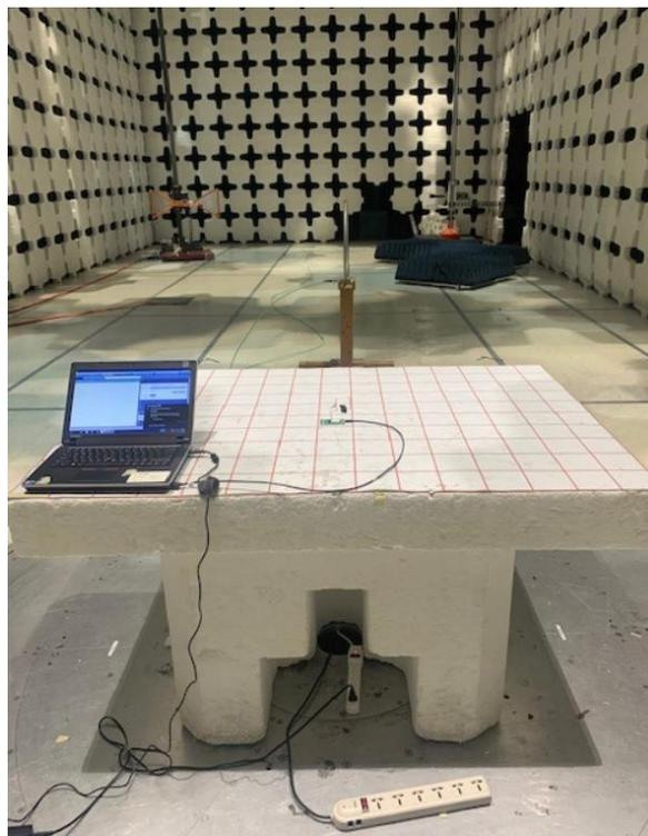
Radiated Emission Test below 30MHz Rear View
