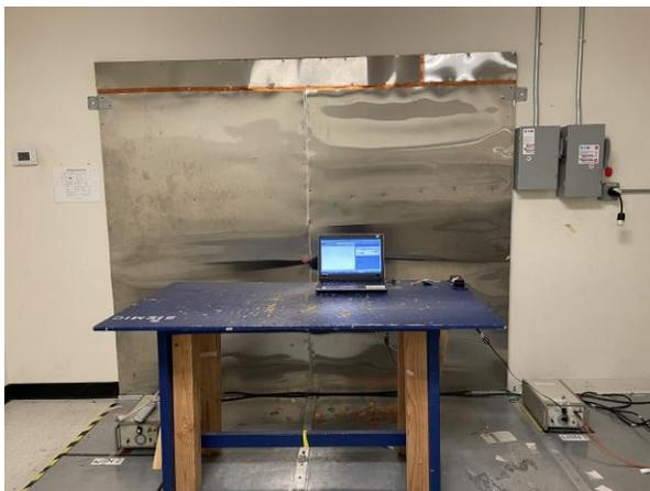
Conducted Emission Test Front View
