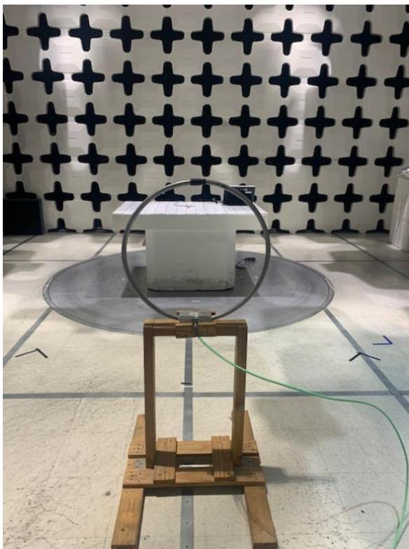
Radiated Emission Test below 30MHz Front View
