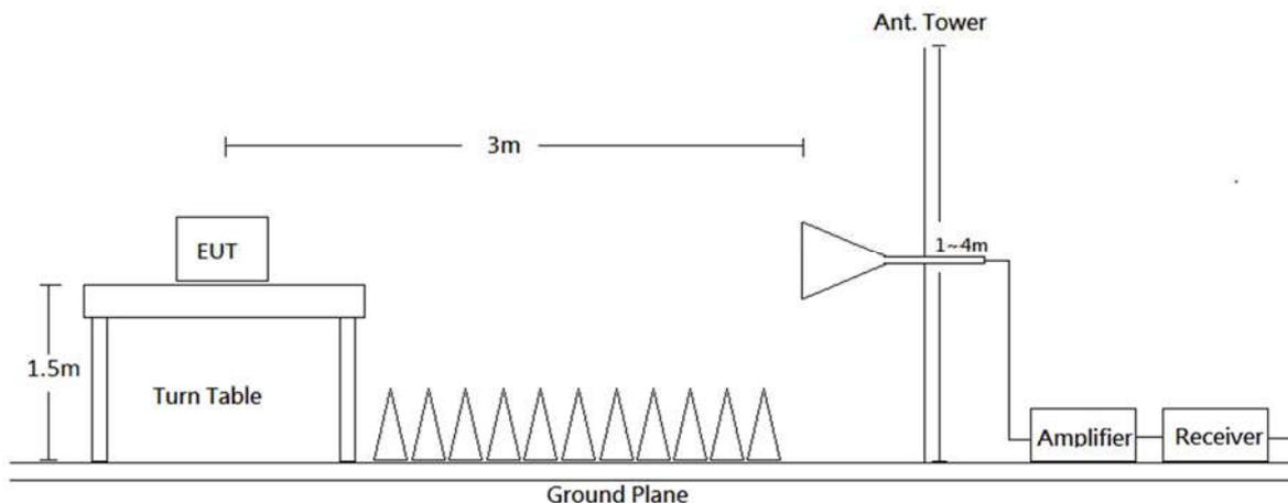
Radiated emission tests were performed in the 3 meters chamber test site, using the setup accordance with the ANSI C63.10-2013. The specification used was the FCC Part 15.209, FCC 15.247 and RSS-Gen, RSS-247 Limits.
