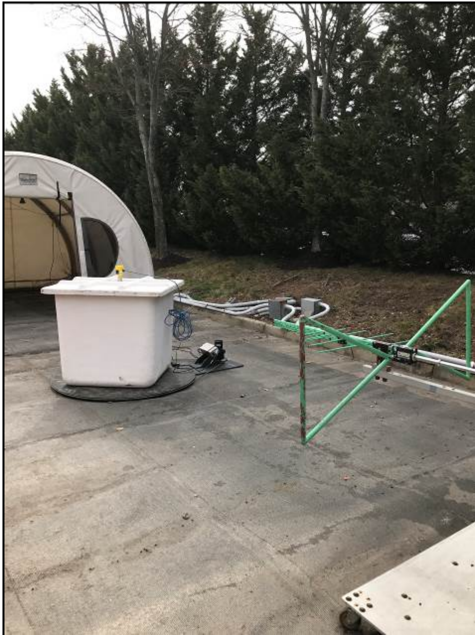
Photograph 19: Radiated Emissions – TC #3; Fiberglass Container
