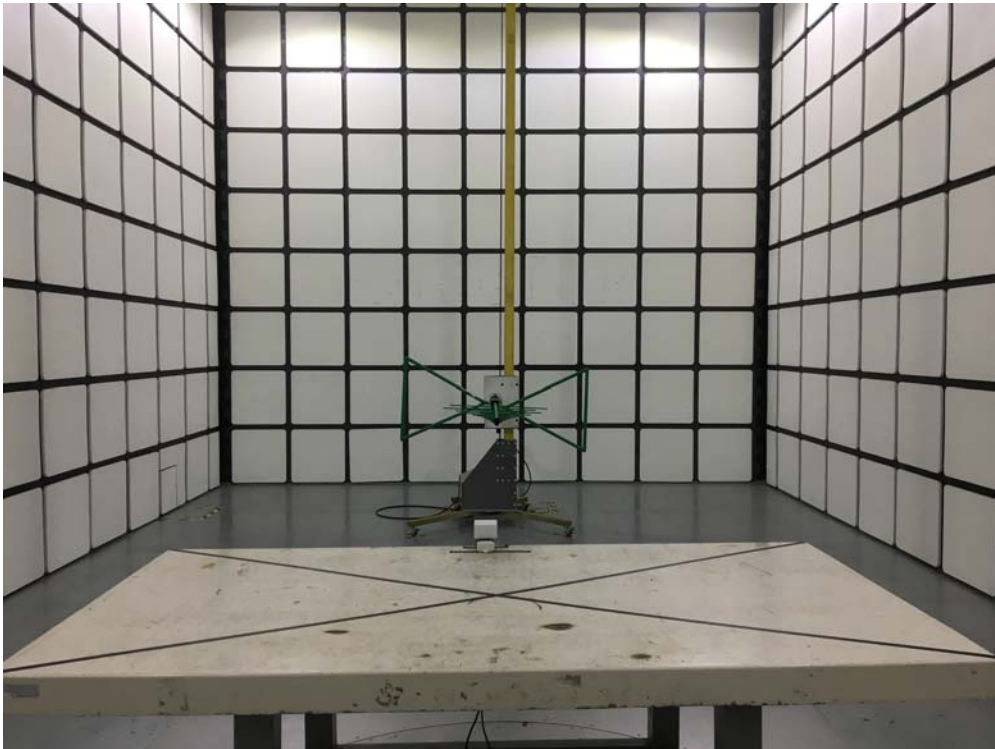
Description: Radiated Emission Test Setup for 1~18GHz
