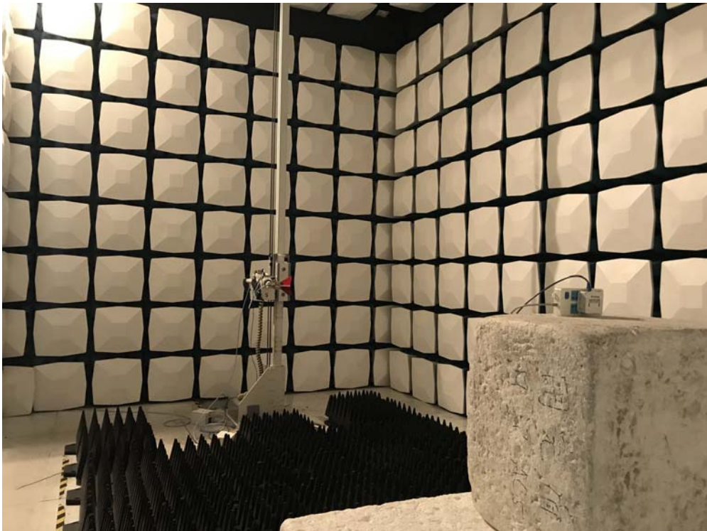
Description: Radiated Emission Test Setup for 1~18GHz
