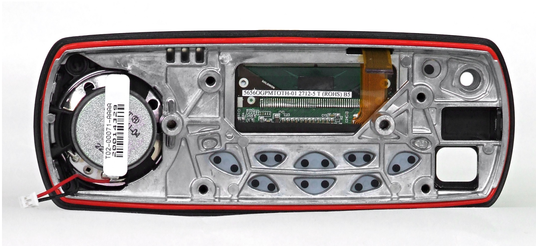
Photograph 06: Control Head – Internal with main PCB removed
