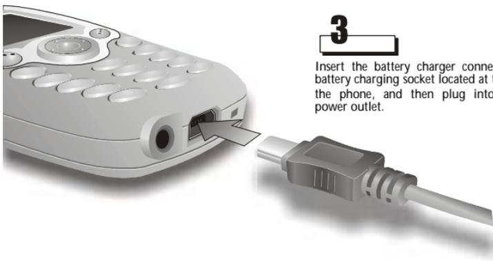
Insert the battery charger connector into the battery charging socket located at the bottom of the phone, and then plug into the electric power outlet.
