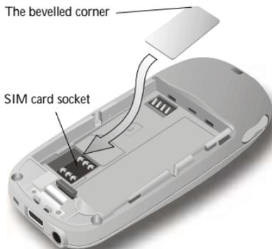
Pay special attention to the SIM card when you install. The metal contacts can be damaged easily by scratches.
