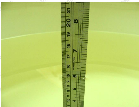
Photo of Liquid Height for Body SAR
