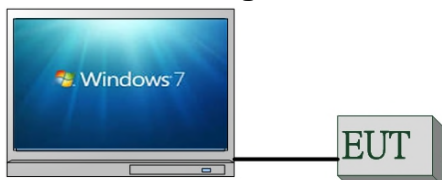
Fig. 2-1 Conducted (Antenna Port) Emission Configuration
